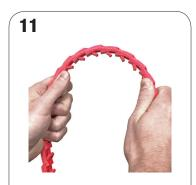
Rotate assembled belt so tabs are inside (facing down into the pulley groove).
