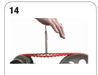
Using a force deflection gauge, check Installation force and confirm it meets the requirements below.
