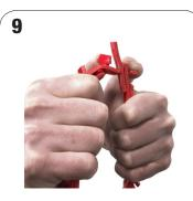
With your thumb twist second tab 90°. Push belt end down over tab with your opposite hand. For wedge profiles, repeat with remaining tab.
